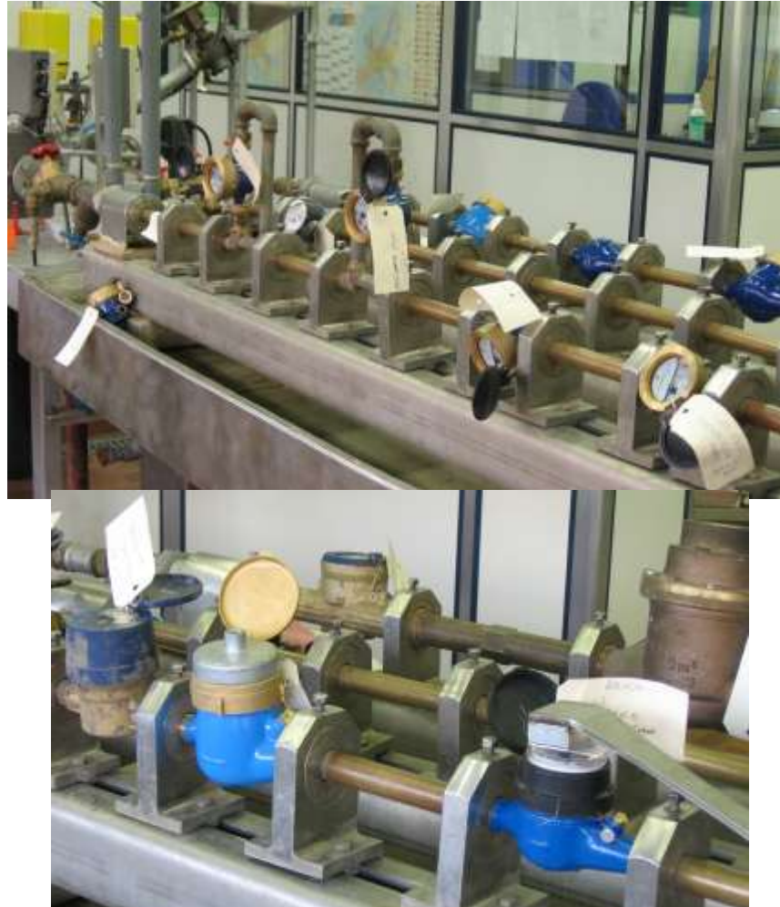
Figure 7 : Water meters on the LECE test bench during the tests
