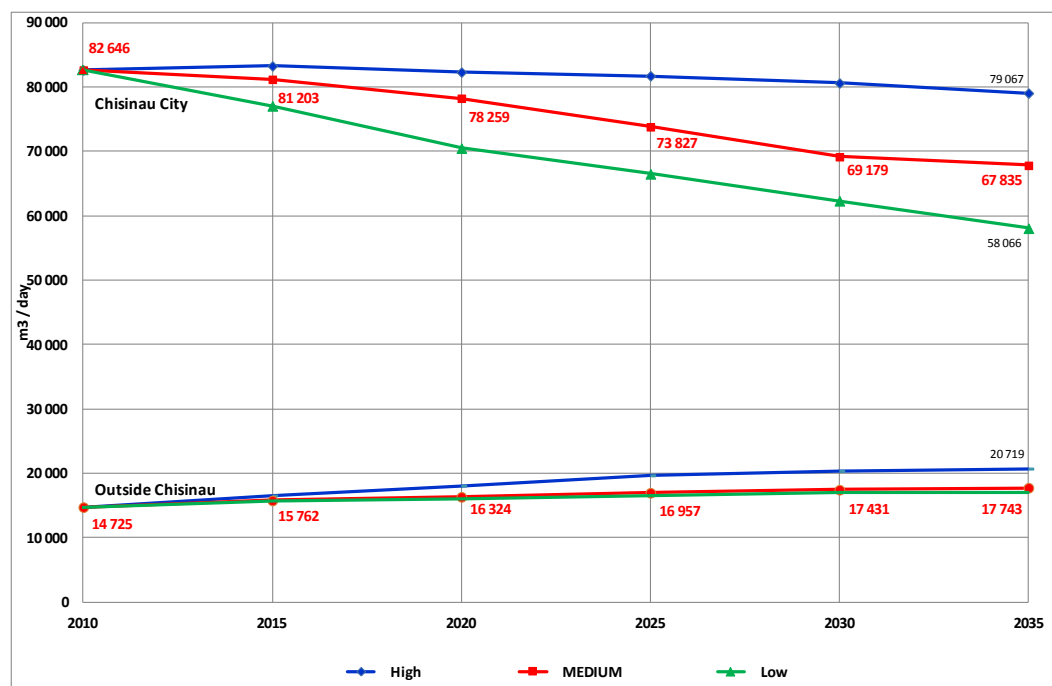
Figure 29 - Domestic water demand per broad geographic area: evolution 2010-2035, according to 3 assumptions (m 3 /day)
