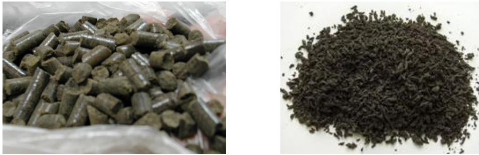
Figure 18 Dried sludge under granulate (left) and pelletized (right) forms
