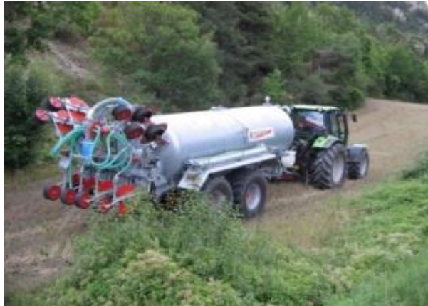
Figure 33 Equipment for sludge spreading on agricultural land
