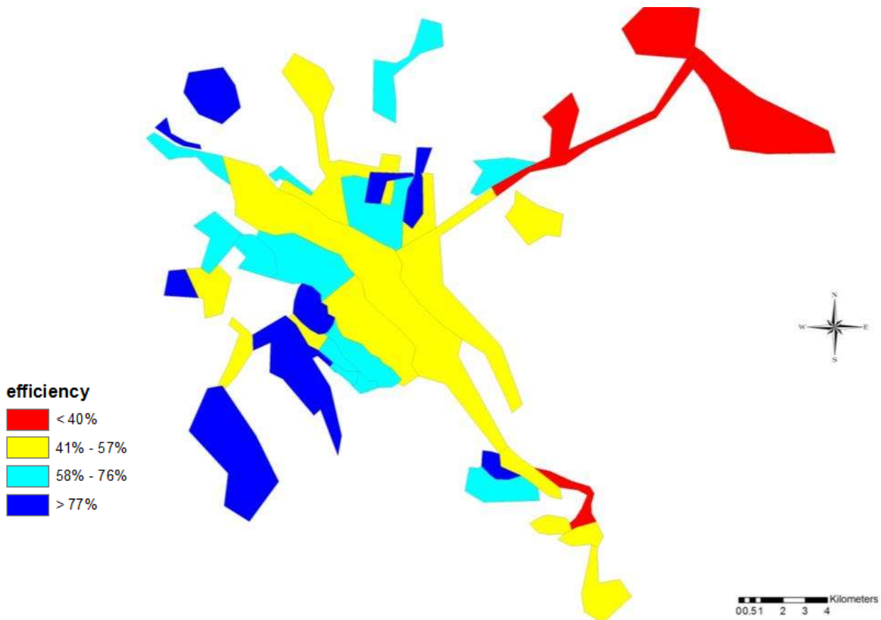
Figure 1: Network efficiency for all the hydraulic entity
