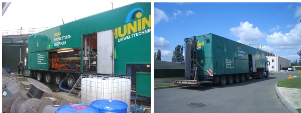
Figure 10: Photos of the equipment to be used for the sludge dewatering tests
