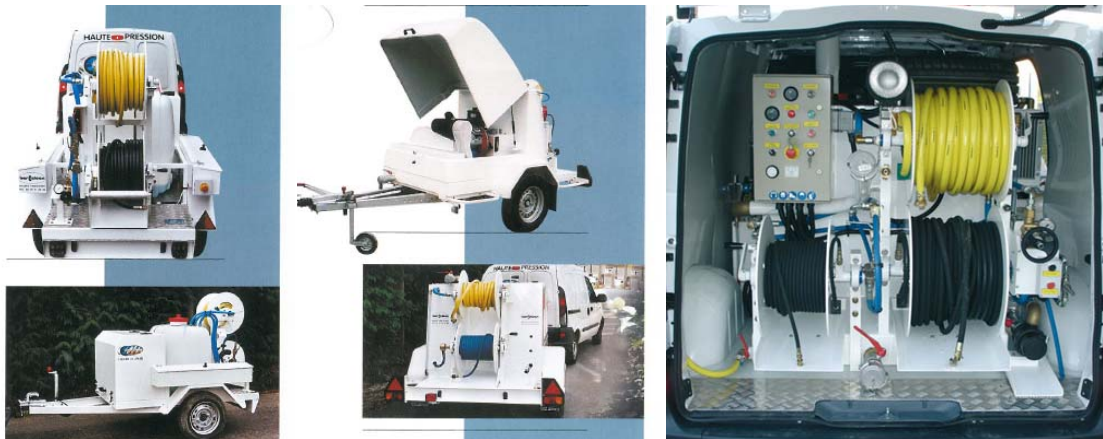
Figure 4-19: Jet unit on trailer or embarked
