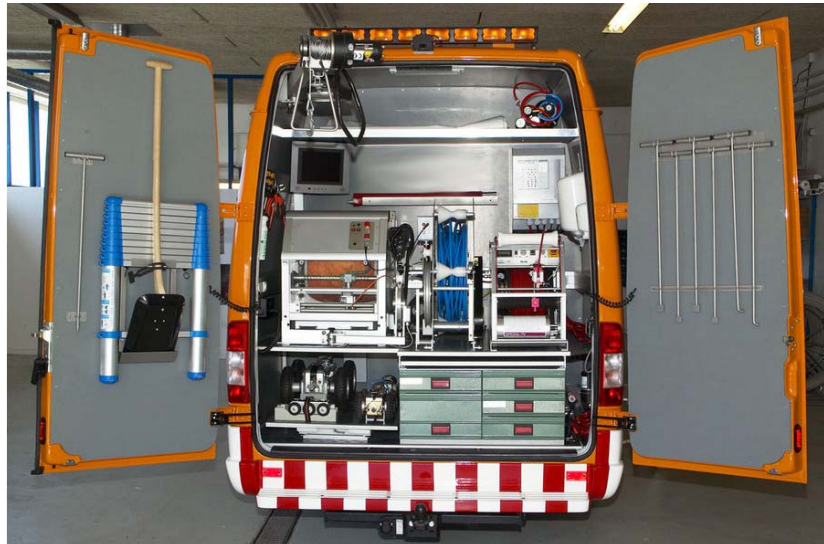
Figure 4-16: Typical CCTV inspection truck 21
