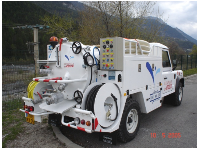
Figure 4-21: Hydro vacuum combination unit on truck
