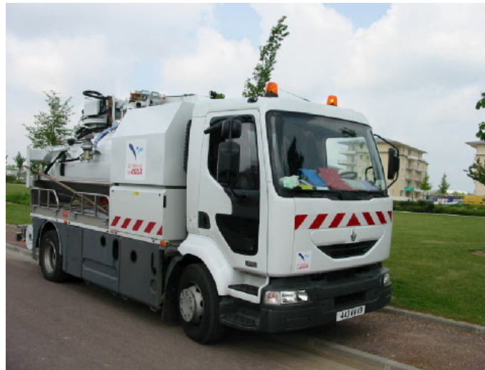
Figure 4-21: Hydro vacuum combination unit on truck
