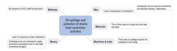
Table 10: Analysis of a drain contamination through 5 M's
